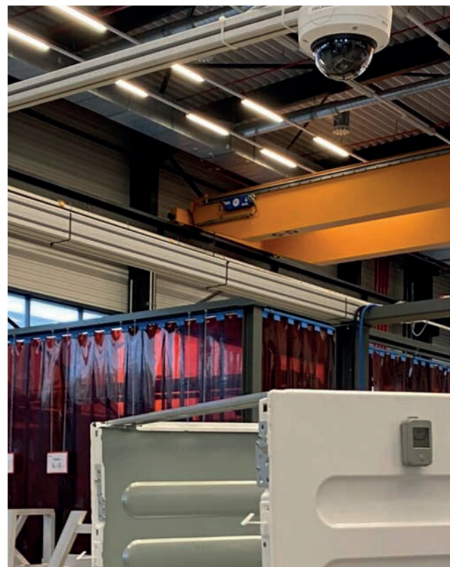
Image 1: Identification and Localization of Components Using Bluetooth Low Energy Beacons and Recording of Processing Operations via Camera Systems Combined with Artificial Intelligence
